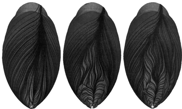
Fig. 5 Oil flow for \alpha = 62 deg and \beta = 20 -deg case. the windward side is larger in the tab case, whereas the strakes act more to even out the regions. Plus, the high-energy vortices from the strakes provide a stabilizing influence over the bump asymmetry. This allows the effect of the sideslip angle, not the physical imperfection, to control the yawing moment. The effect of these control devices on the static pitching moment has to be considered along with their impact on lateral directional stability. At sideslip angles any increase in nose-up effect can be detrimental. The strake does an extraordinary job of limiting an
